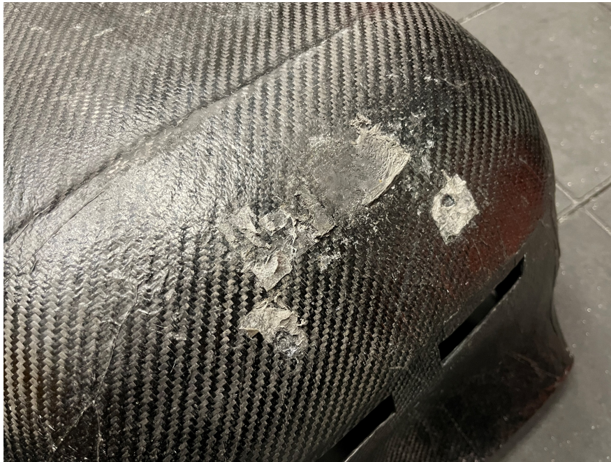
Figure 39 ART_08's CFRP seat bottom abrasion
