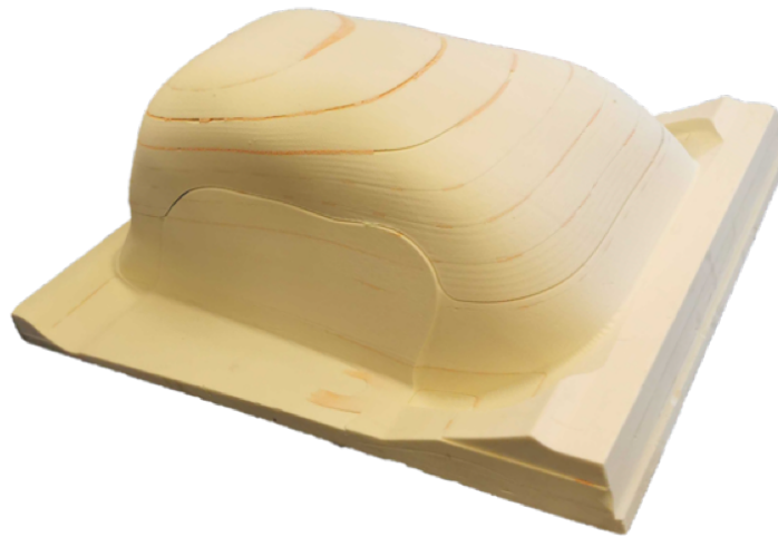
Figure 24 ART_08 seat mold after milling
