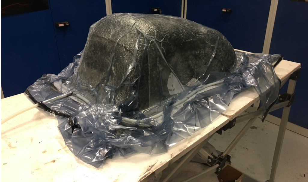
Figure 30 ART_08 CFRP seat during manufacturing
