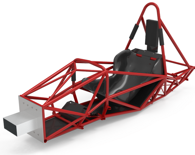
Figure 10 Render of ART_07 tubular steel spaceframe assembly
