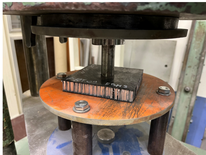
Figure 16 Perimeter shear test
