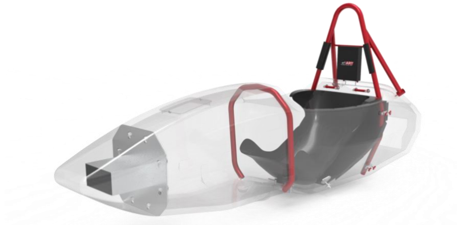
Figure 12 Render of ART_08 monocoque chassis assembly
