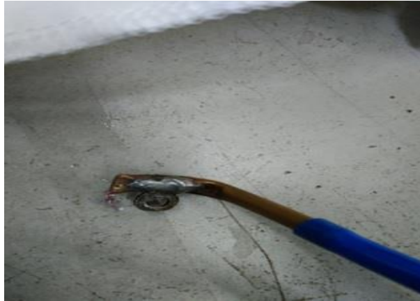
Figure 7: Air Flowing Device Made to Supply Compressed Air
