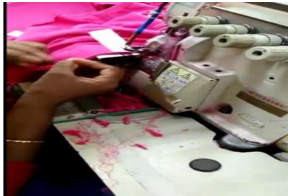
Figure 9: Connection of the Air Flowing Device with the Presser Foot of the Machine
