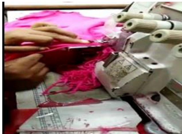
Figure 5: An Example of Generated Sewing Waste in the Overlock Machine
