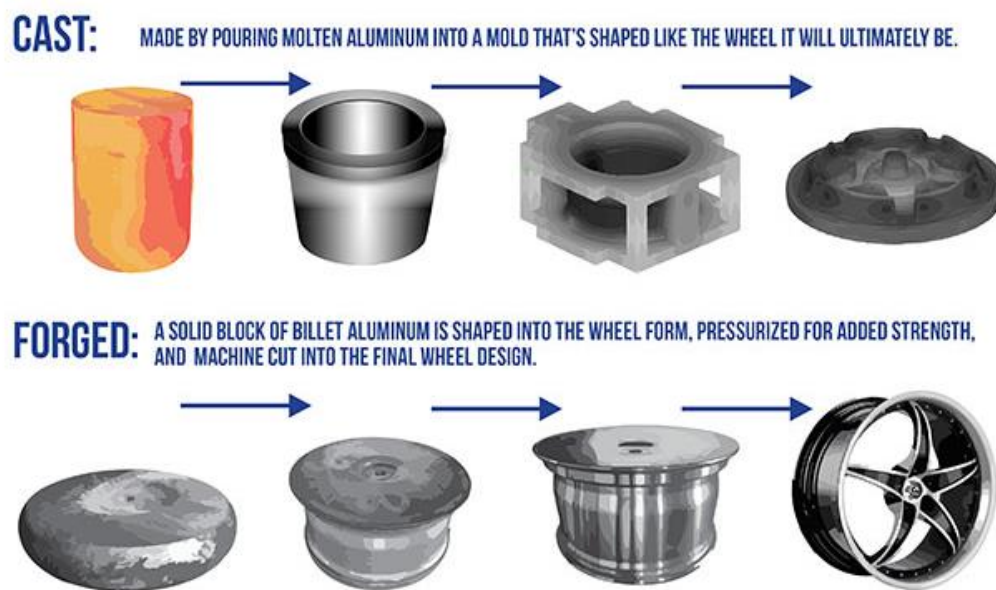
4. Figure Casting and forging processes in wheel manufacturing 4
