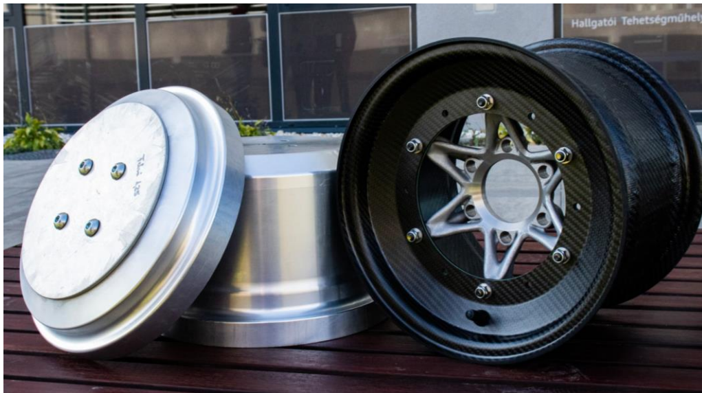
13. Figure The hybrid CFRP wheel used in 2022 and its laminating mold 12
