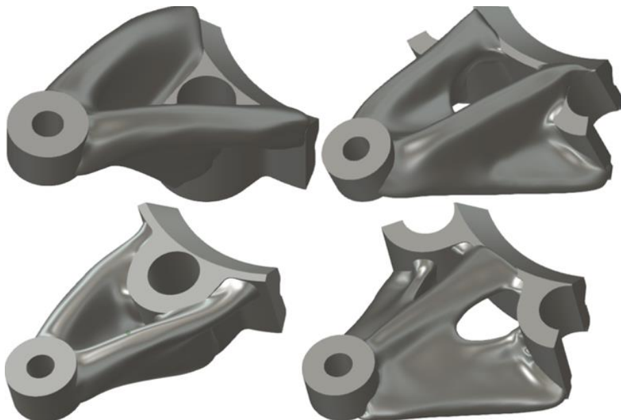
41. Figure Different machinable center geometries made with generative design
