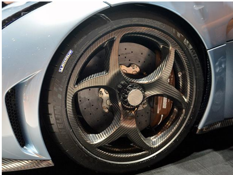
6. Figure Koenigsegg Regera's CFRP wheel 6
