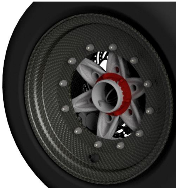
39. Figure The new wheel center in the wheel assembly
