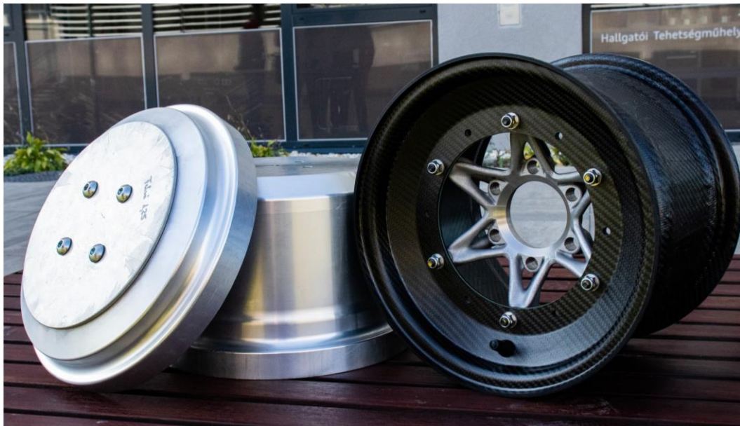
12. Figure The hybrid CFRP wheel used in 2022 and its laminating mold
