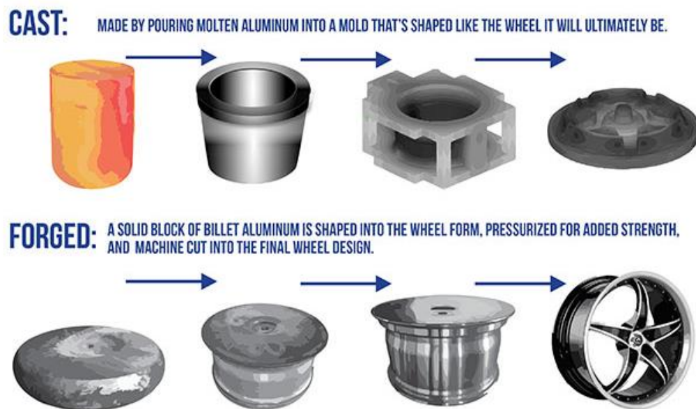
4. Figure Casting and forging processes in wheel manufacturing 4
