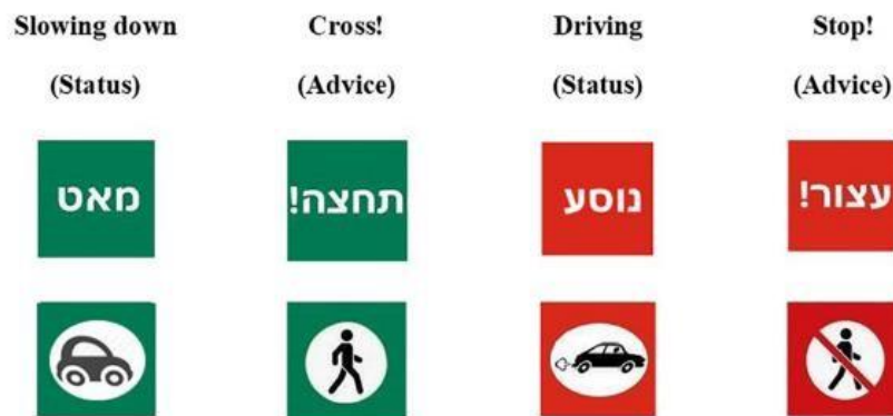
FIGURE 3 | The e-HMI Messages; each column displays the message type (status or advice) in both written (in Hebrew) and symbolic messages. The background color is compatible with the message meaning according to the color convention.
