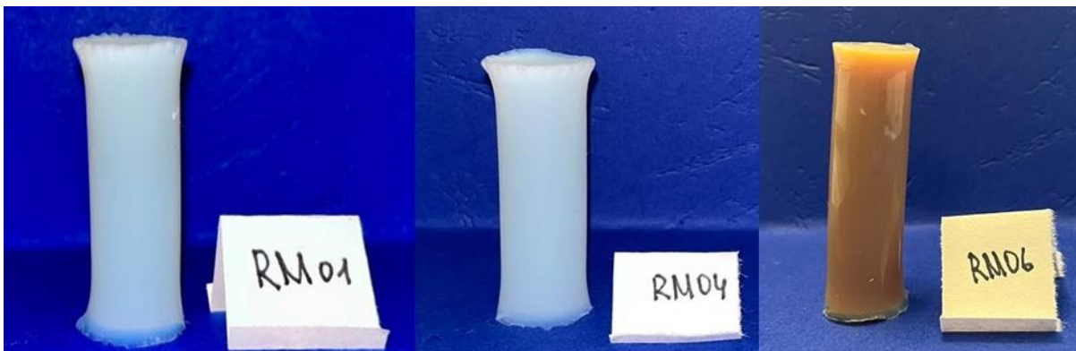
Figure 7. Pictures of freshly synthesized aerogels with their identity codes
