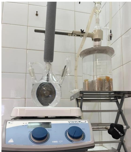
Figure 6. Solvent regeneration and extraction unit
