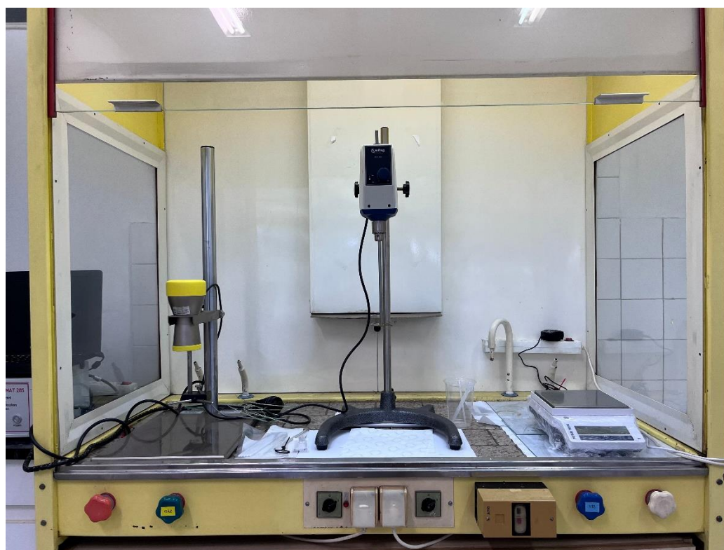
Figure 3: Foam Qualification System FOAMAT 285
