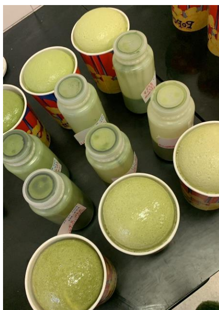
Figure 7: Freshly made polyurethane foams with algae
