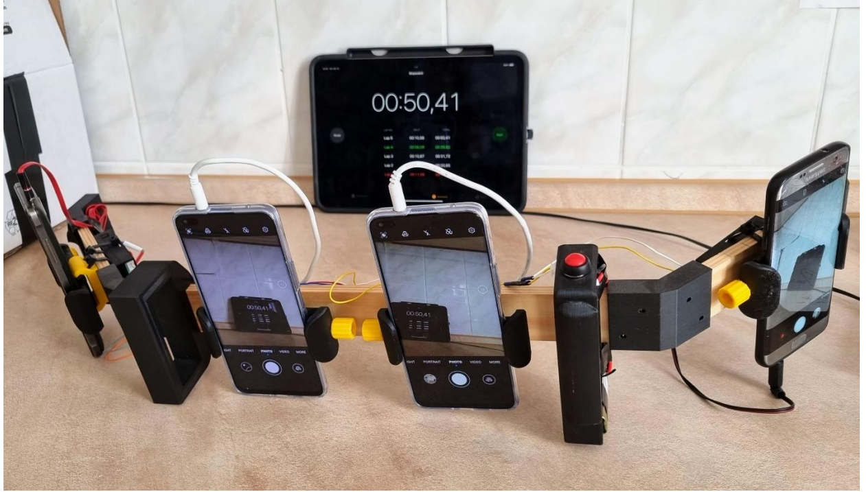
Fig. 16. Testing the release lag between the cameras.
