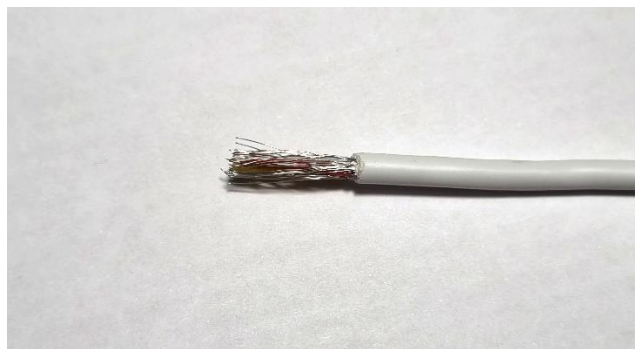
Fig. 3. The external insulating layer removed.
