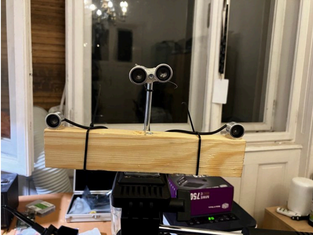
Figure 5: Ultrasound locator test setup. The two receivers on the wooden part are 20 cm apart from each other; the third receiver is 6 cm higher to the other two. In the center the left one is the receiver; the right is the transmitter.
