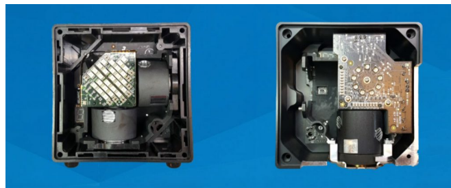
Figure 5: first-generation lighthouse internals (left) and second-generation lighthouse internals (right) [1]
