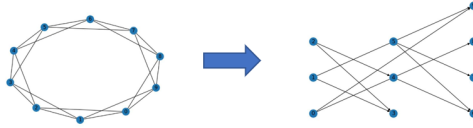
Figure 5: Illustration of the conversion of a WS network to a directed acyclic graph.
