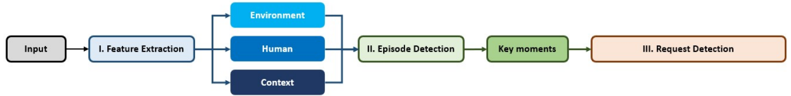
Figure 4.1: Overall Composite AI framework with three main modules: feature extraction, episode detection, and request detection.
