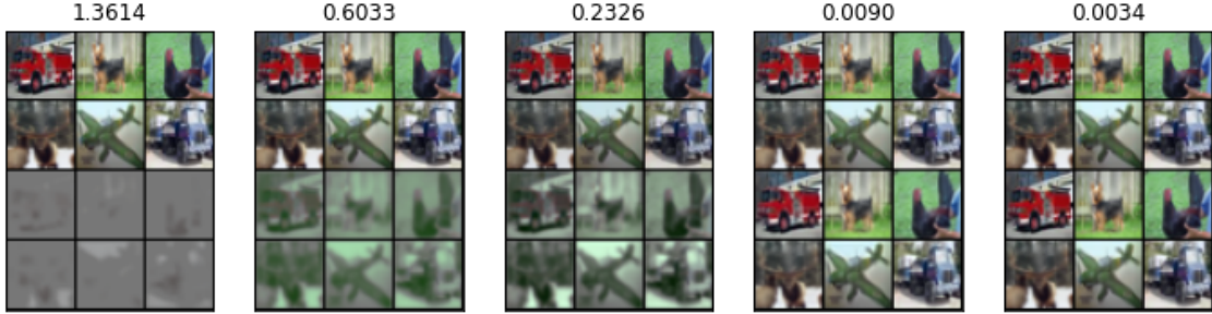
Figure 2.2: Examples of different reconstruction loss values. The top two rows of each block are the original images and the bottom two rows are their reconstructed versions. The reconstruction loss of each case is denoted above them.
