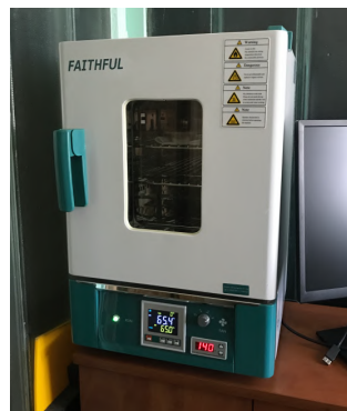
Figure 4.9: The curing process in the drying chamber
