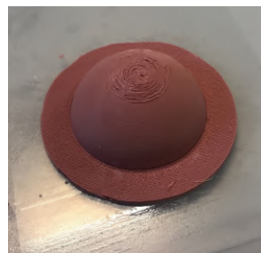
Figure 4.10: The final silicone shell
