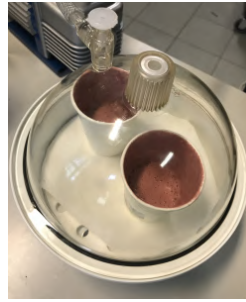
Figure 4.6: Degassing the silicone in the vaccuum chamber
