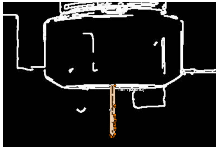
Figure 7 - Annotation sample of smaller tools. The width of the tool is so small (1 mm) that Canny edge detection fails to correctly identify the edges, causing the tool to appear as a single edge.
