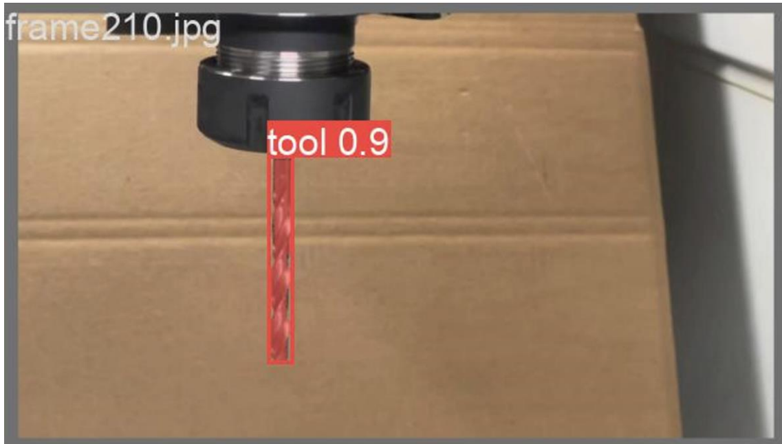
Figure 12 - Model predictions showing issues with edge identification in frame210.jpg.
