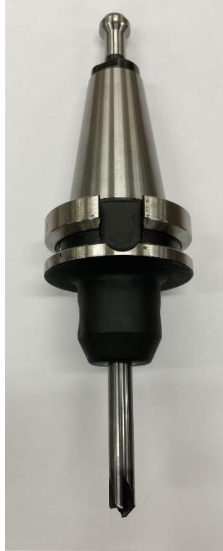
Figure 16 - A chamfer making tool with an edge fracture.
