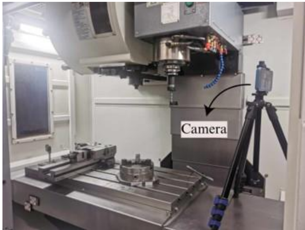
Figure 3 - Camera and tripod inside the CNC cabin.
