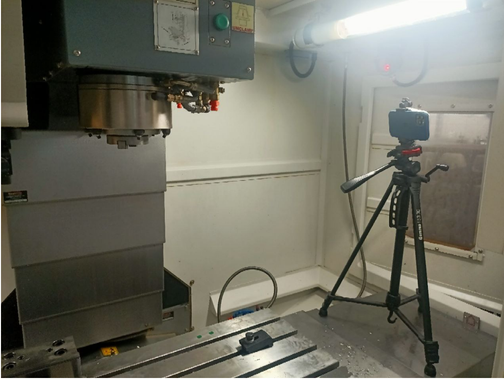
Figure 3.1: Camera and tripod inside the CNC cabin.
