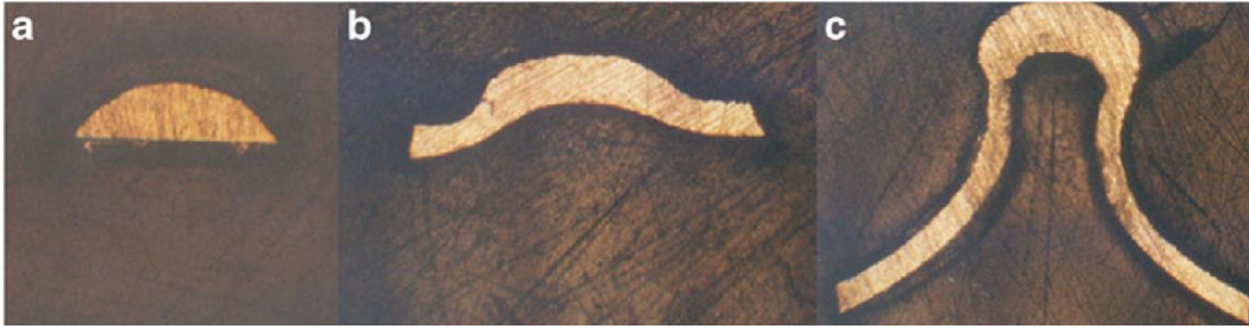
Figure 7: Cross-sectional geometry of thread chips: a. First pass, b. Intermediate pass, c. Last pass [23]
