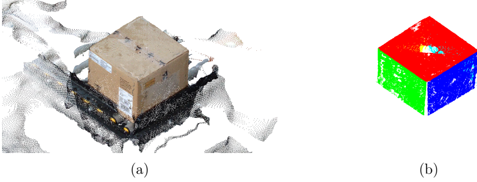
Figure 4.9: (a) The original point cloud before the planes are segmented. (b) the result of five segmented planes.
