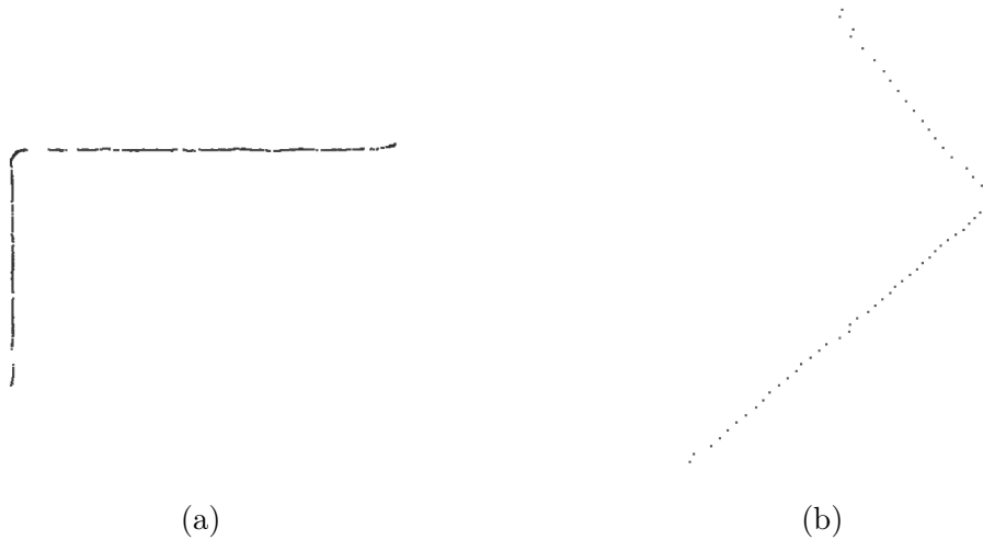
Figure 4.8: (a) Sampled point cloud from the depth camera after transformed into 2D. (b) 2D LiDAR points before alignment with the sampled points.
