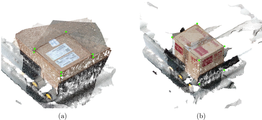
Figure 5.5: Corners extraction in relatively (a) thin and (b) small boxes.
