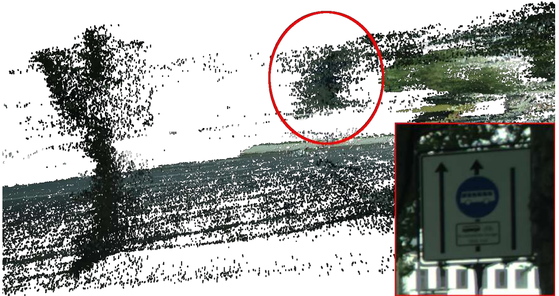
Figure 4.3: Side view of pointcloud generated from disparities (Cityscapes dataset). The points of the sign in the bottom right corner are circled in the center. As errors affect the depth of the points more, the pointcloud is distorted, the signal to noise ratio on the surface is very low. This makes the detection of surfaces perpendicular to the viewing direction particularly challenging.
