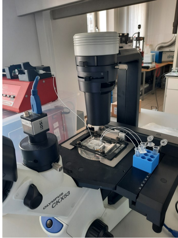
Figure 3.10: The assembled working platform. On the left side is the syringe pump on an elevated platform, the device is on the microscope and the outlets are placed in centrifuge tubes.
