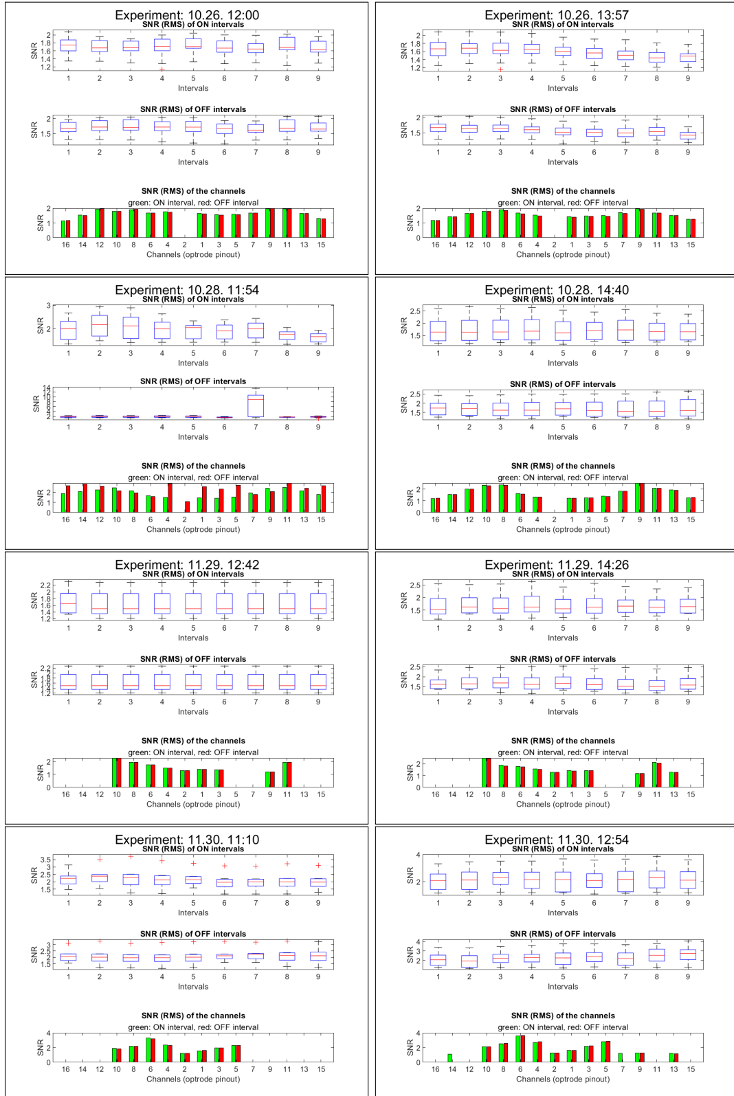
Figure 7: The summary of the RMS-based signal-to-noise ratio values. To provide a comprehensive analysis, each plot displays data for 9 intervals of IR stimulation, alternated with periods of rest (ON and OFF respectively). The first two plots contain SNR values for the ON and OFF intervals, respectively. The third plot shows the SNR values for individual channels for the ON (green) and OFF (red) IR stimulation intervals.
