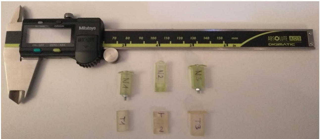
Figure 14: Micro-drive components for the water test. Components labelled with N are printed with Phrozen Nylon-Green Tough 3D Printer Resin, while those labelled T are made from Surgical Guide Resin prints.
