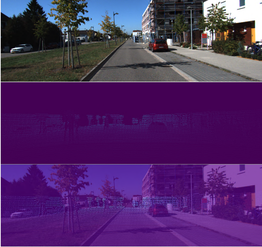
Figure 9: Raw image from the KITTI RAW dataset with the LiDAR ground truth depth converted to an image. These converted images are used for evaluating our models.
