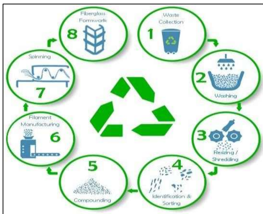
Figure 8. Plastic Products Recycling Process for Fiberglass Formwork (Edited by the authors)
