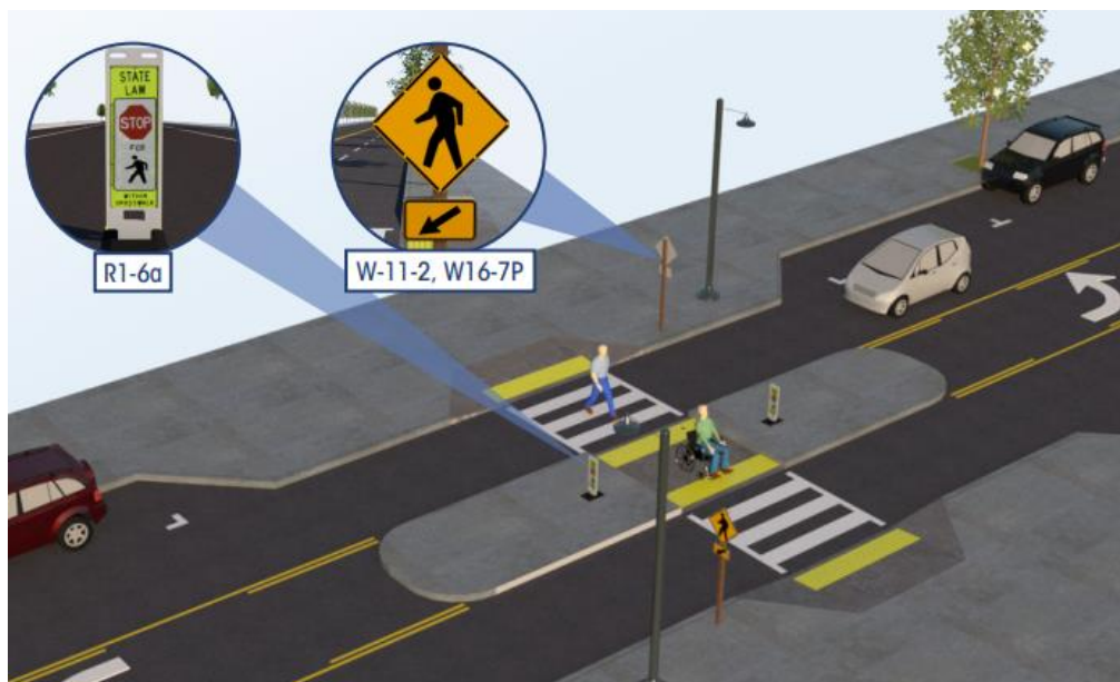
Figure 4: Refuge Island Design with Reflective Signs and Mounted Signs.
