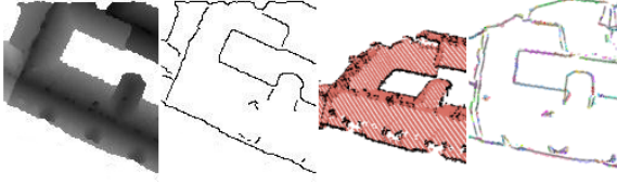
Figure 3: Outer edge detection's assembly - projection (z-image) - edge detection - elevation into the 3D space - segment fitting.
