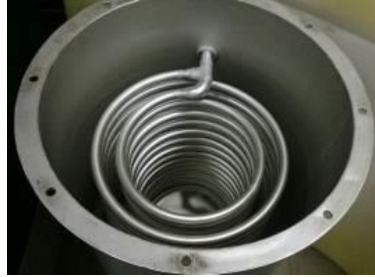
Figure 4 The double pipe coil inside the tank
