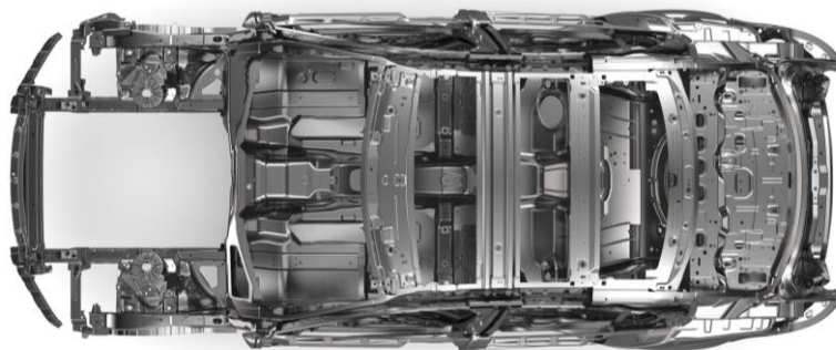
Figure 4.: More than 2400 Self Pierce Rivet joins in the Jaguar XE
