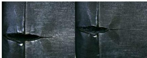
Figure 14 Chip injuries on the rollers II.
