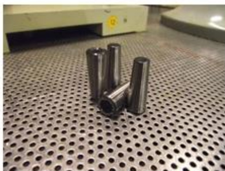
Figure 7 Finished rollers (left) and grinded rollers (right)
