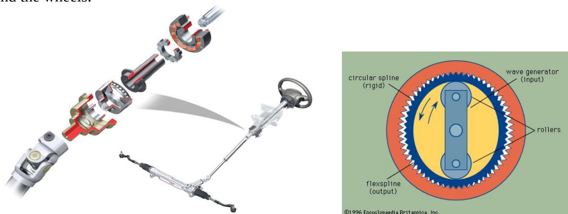
Figure 2 AUDI steering unit with harmonic drive [1]
