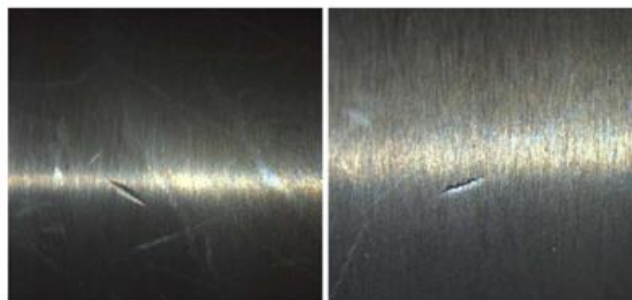
Figure 16 Dents on the rollers due to mishandling
