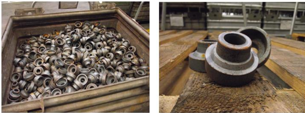
Figure 1 Raw material (left) and tower rings (right)
