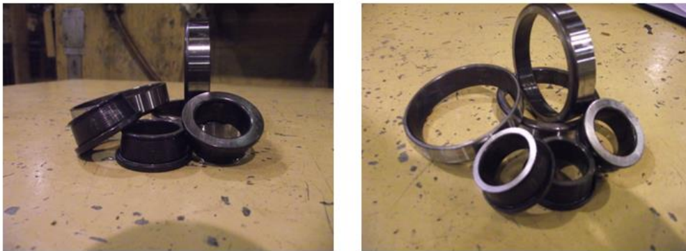
Figure 4 Side grinded rings (left) and lateral surface grinded rings (right)
