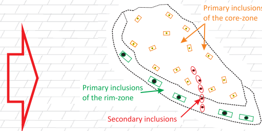
Fig. 8. Sketch of the observed co-genetic hydrocarbon and aqueous inclusion generations. Any co-genetic aqueous inclusion was not found along secondary inclusion assemblage.
