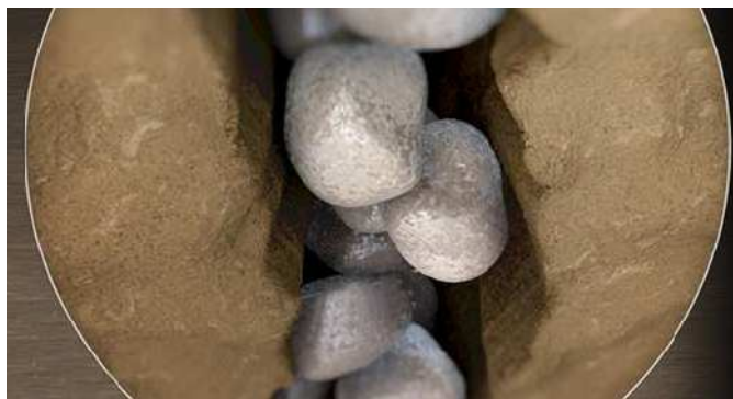
Fig. 1: Proppants in fracture
