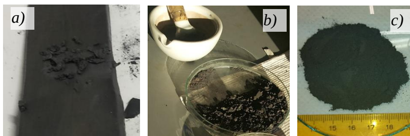
Fig. 2 Collecting (a) and mechanical preparation (b) of the anode slime raw material (c).
