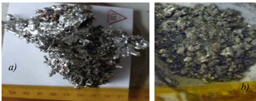
Fig. 1 Picture of the broken soldering waste material (a) , dross (arose from the melting of the metal in air) (b).
