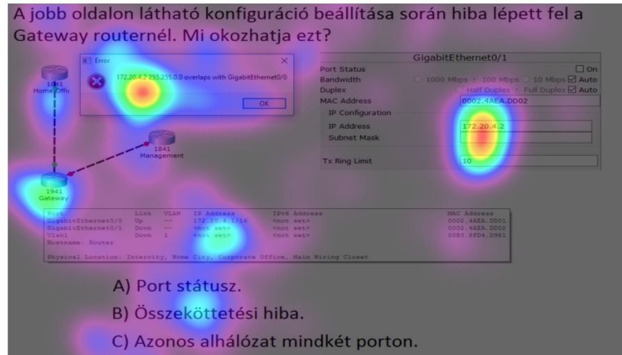
Fig. 12 Gaze path, fixations and connections when one of the users reading the task
