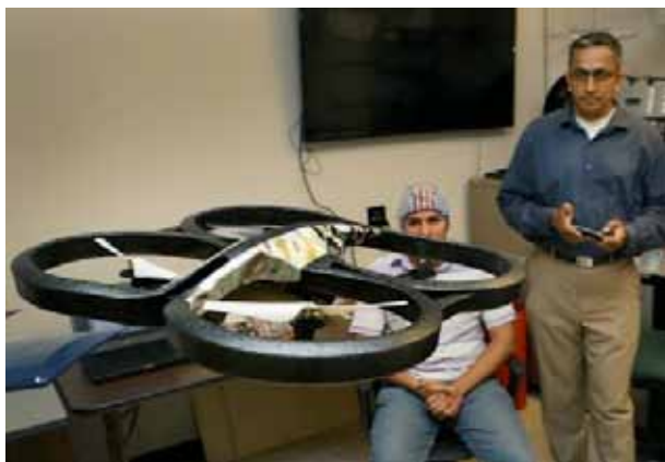
Figure 7. A helicopter controlled by brain waves.
