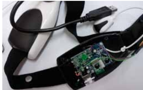
4. Figure. Joining the USB UART transformer and the MindFlex headset.
