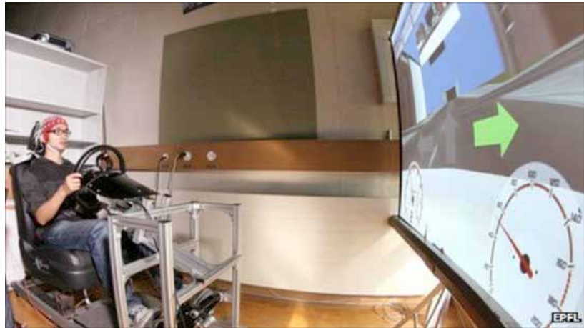
6. Figure. A system that helps the braking based on brain wave perception.
