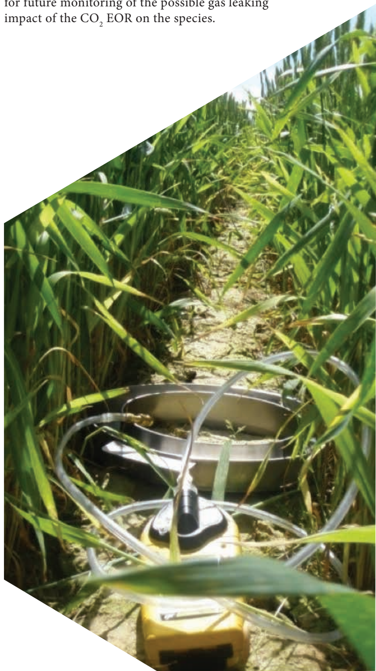
Fig. 8. Application of gas detector on the site
