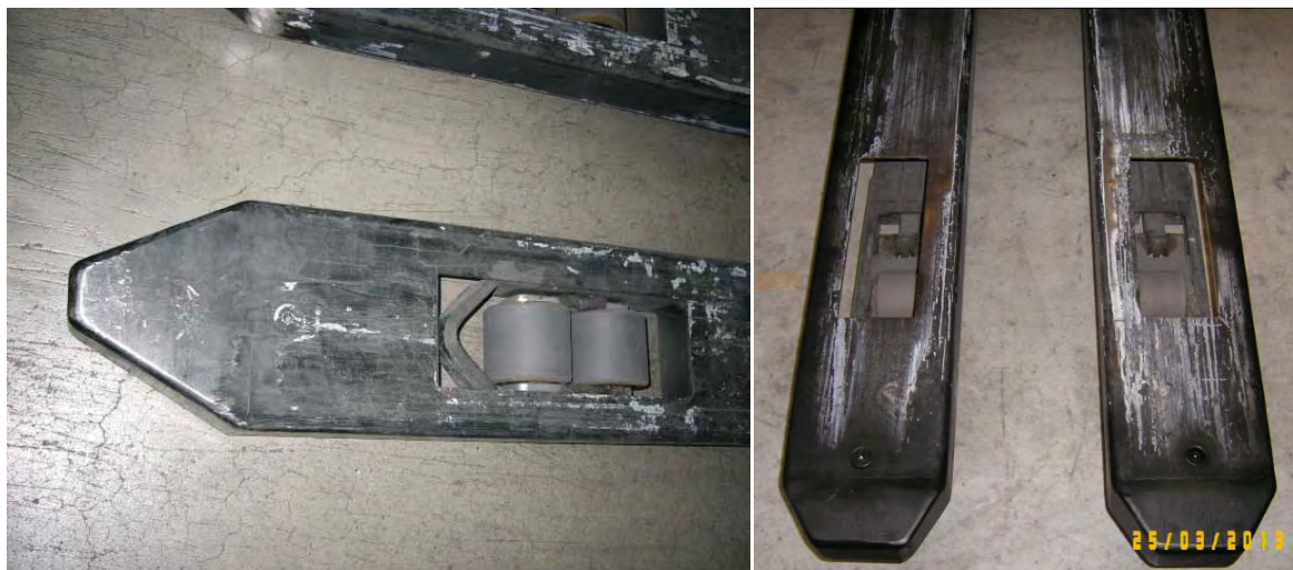
Obr. 12 Vidlice pred a po oprave Fig. 12 Forks before and after repair
