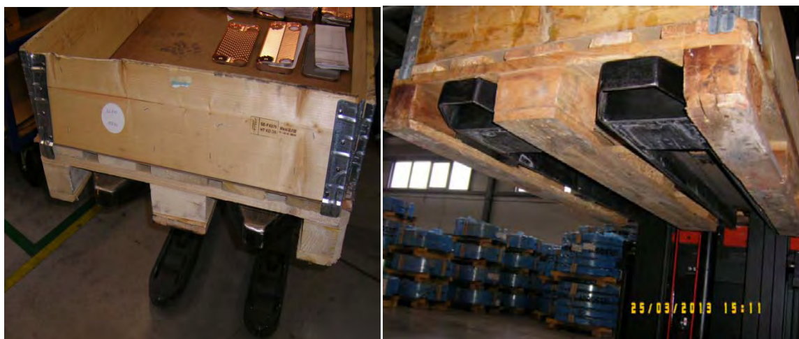
Obr. 11 Vidlice pred a po oprave Fig. 11 Forks before and after repair
