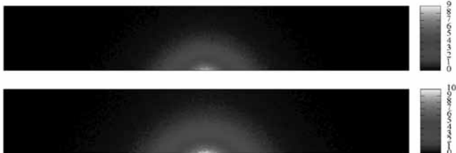
Figure 1: Ratio of successful docking as a function of the initial position and the effect of ambient temperature, 40 °C (upper), 60 °C (lower).
