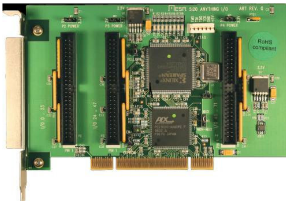
2.1. Figure: Mesa electronics 5i20 I/O PCI Card
