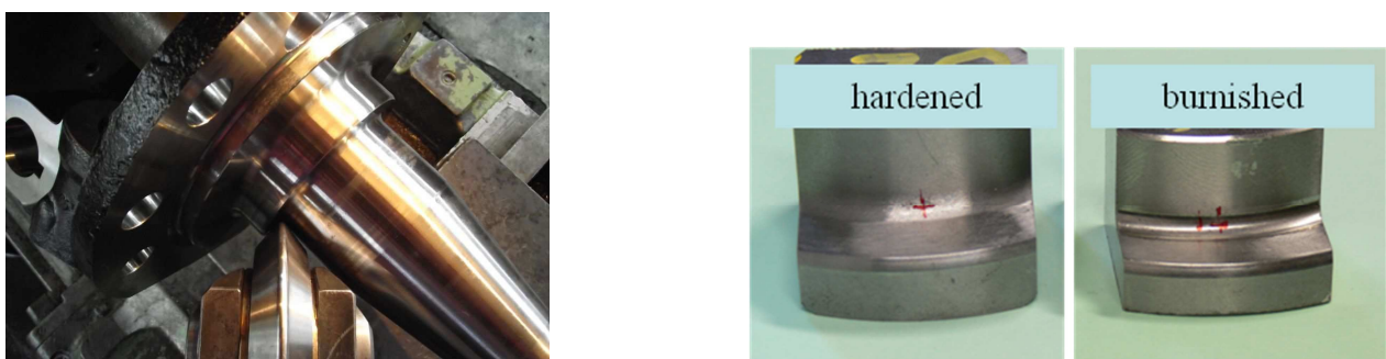
Fig. 4. Experimental setup of roll burnishing, parts of the hardened and the burnished samples
