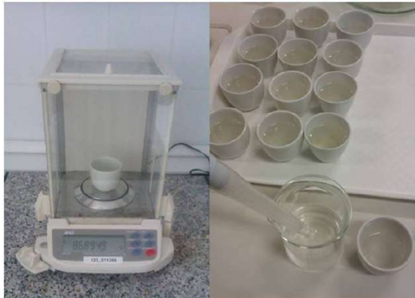
Figure 8.1: Total suspended sediment determination using analytical scale (left.: scale, right: water samples in the cups) (Kutai, 2014)
