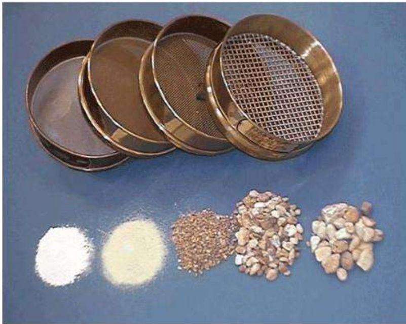
Figure 8.5: Logarithmic sieves for separating size groups
