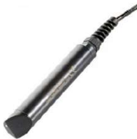
Figure 6.14: Ponsel NTU digital turbidity meter
