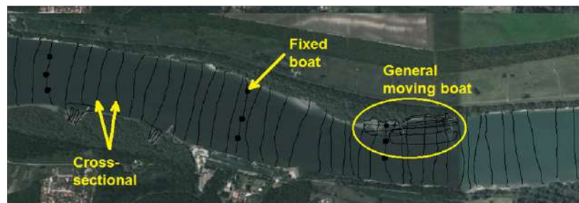
Figure 3.7: Path of ADCP measurements conducted in the Danube in the area of Sződliget.
