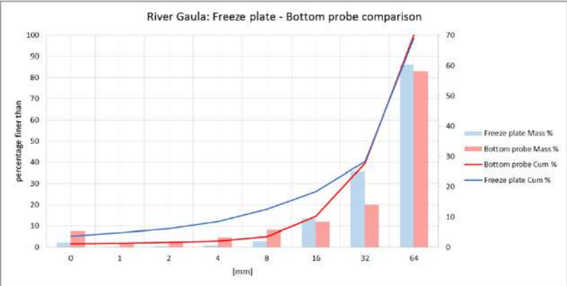
Figure 7.15: Resulting grain size distribution for sample FP1 and BP1
