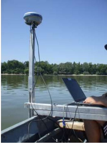
Figure 3.2: RTK-GPS and data recording computer.
