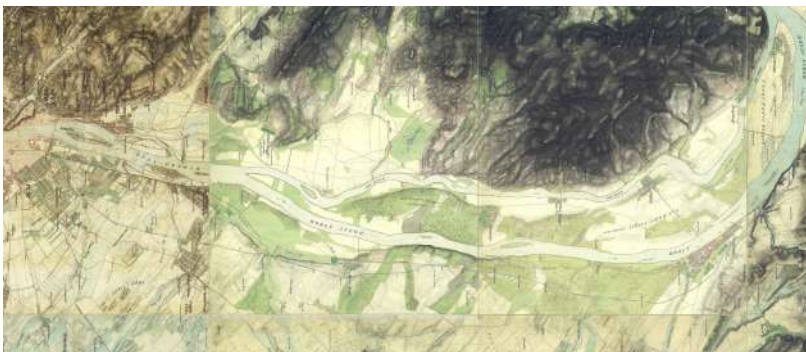
Figure 10.4: The Danube River, section upstream of Budapest, a very nice example of the anabranching planform. The channel has moderate curves and a lot of islands and anabranches can be seen. Vegetation covers the banks, the islands are slowly moving downstream, however the system is quite permanent.
