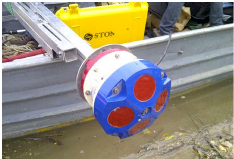
Figure 3.1: Four-headed ADCP device.
