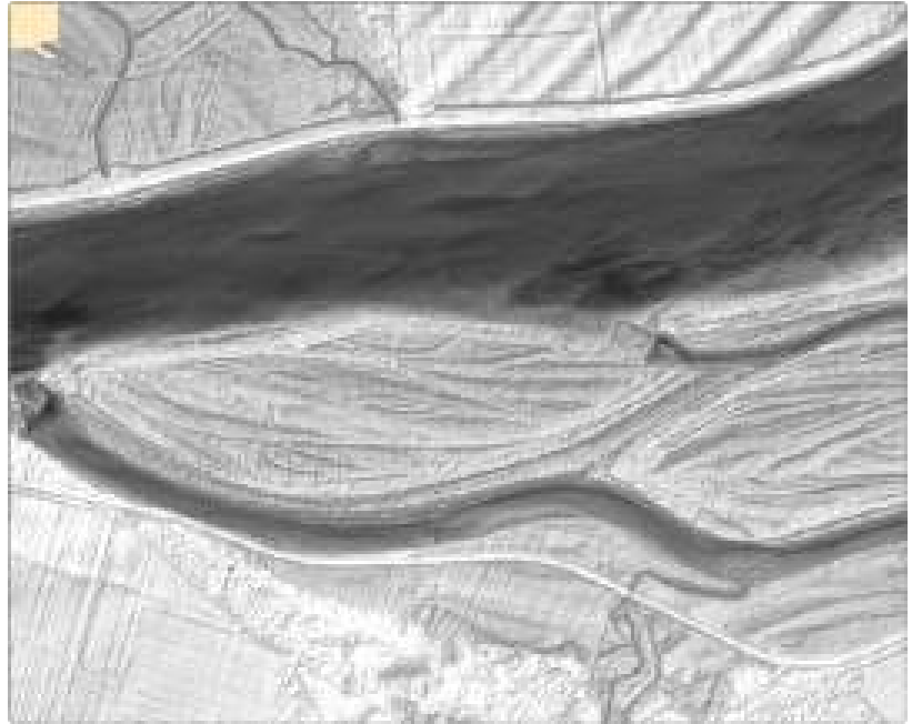
Figure 4.3: Complex terrain map of the floodplain created by ALS LiDAR
