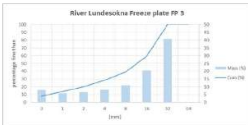
Figure 7.14: Resulting grain size distribution for sample FP 3
