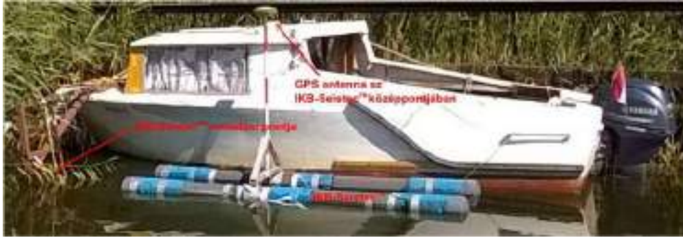
Figure 9.5: IKB-Seistec™ single-channel seismic profiler next to the survey vessel
