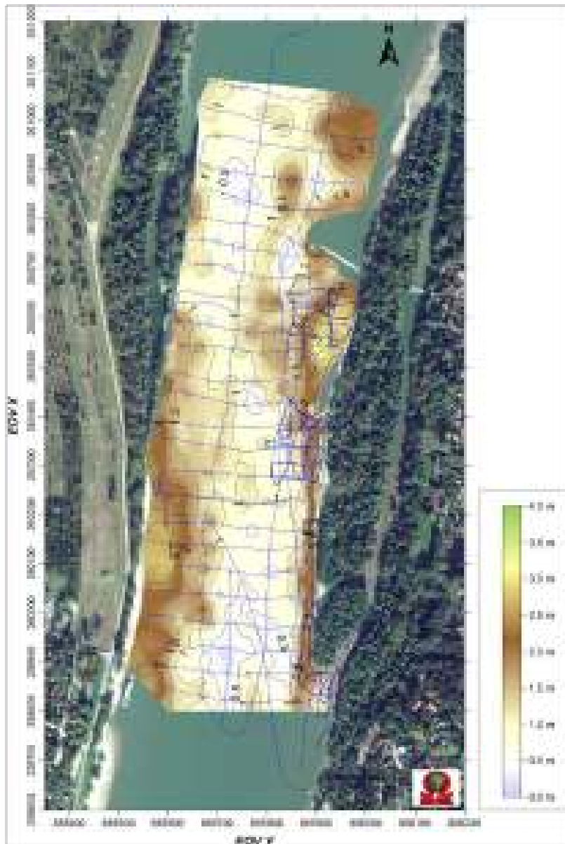
Figure 9.9: Thickness of recent fluvial sediments at Göd-island, river Danube
