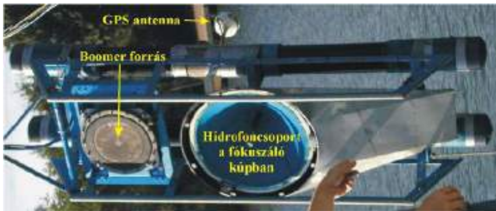
Figure 9.4: Bottom view of the IKB-Seistec™ single-channel seismic profiler
