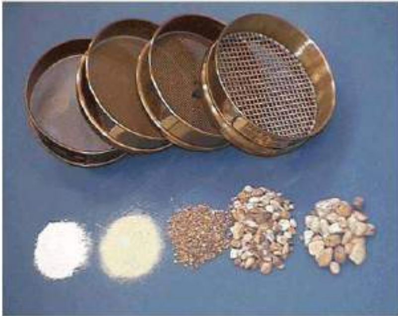
Figure 8.5: Logarithmic sieves for separating size groups
