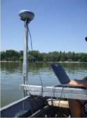
Figure 3.2: RTK-GPS and data recording computer.
