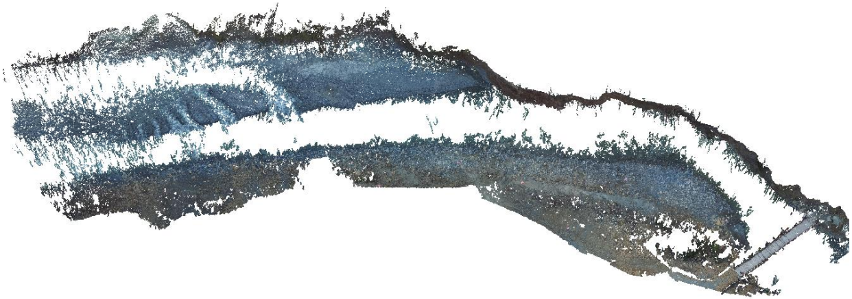
Figure 8. 3D point cloud in VisualSFM of a 300 meter long river reach
