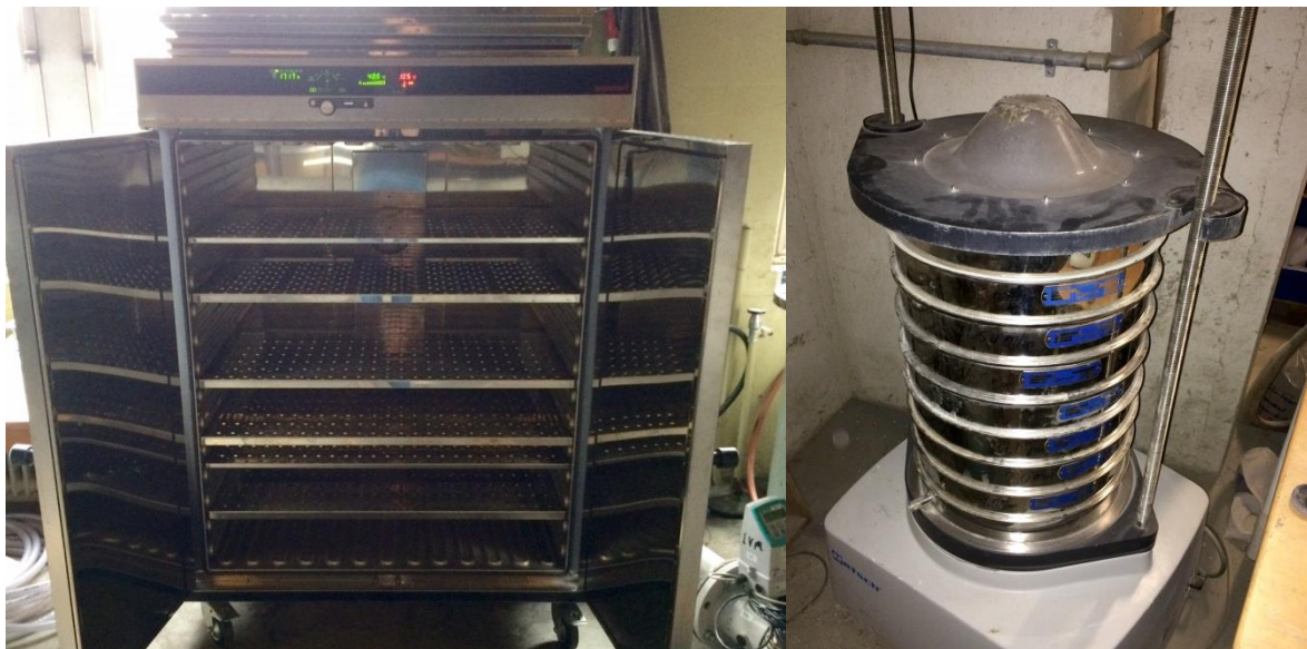
Figure 1. Used oven (left) and sieving machine (right) in the NTNU laboratory.
