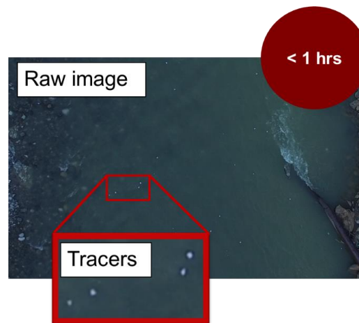
Figure 11. Raw image for LSPIV analysis with tracers on the surface
