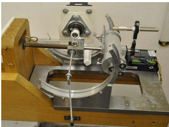
Fig. 3: Setback of the rig, calibration of „zero flexion to zero rotation” state
