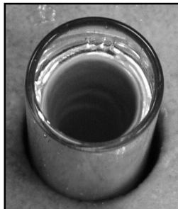
Figure 3. Magnetically stirred liquid Ga-In alloy in D = 14 mm crucible
