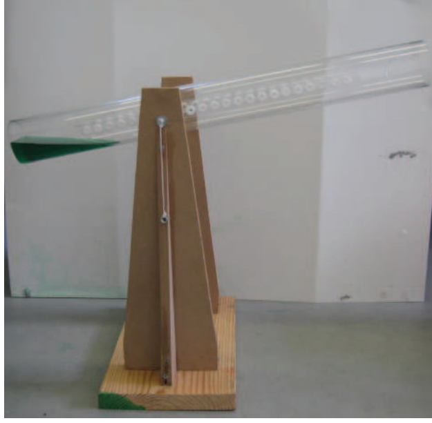
Figure 13: Stable tilt equilibrium of the cylindrical container for the parameters g = 9.8 \text{ m/s}^2 , \rho = 998 \text{ kg/m}^3 , b = 0.92 \text{ m} , d = .095 \text{ m} , p = 0.365 \text{ m} , m_c = 1.38 \text{ kg} , \eta = 0.96 , f = 0.062 \text{ m} , \phi = 81^\circ .
