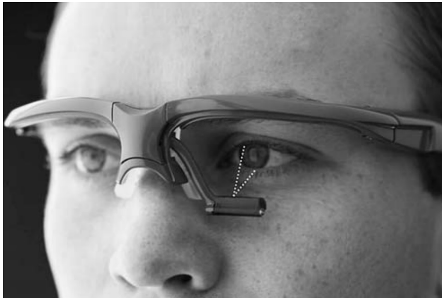
Fig. 3 Spectacleframe recorded oculography based on infrared light reflection
