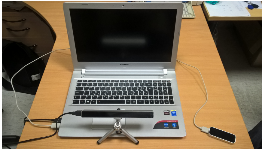
Fig. 7 Test environment with eye tracking and gesture control
