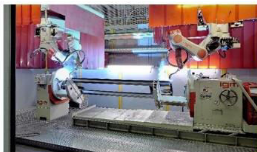
Welding robot system for fork lift masts
