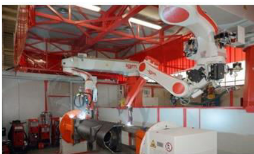
Welding robot system for track roller frames
