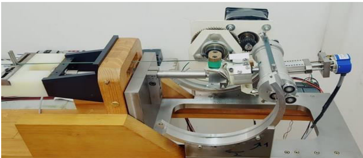
Figure 3 Knee prosthesis test machine.
