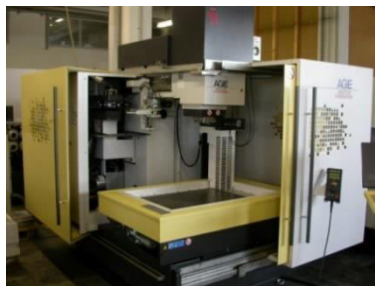
Figure 1 Agietron Hyperspark 3 electro-erosion machine used for the production of experimental samples
