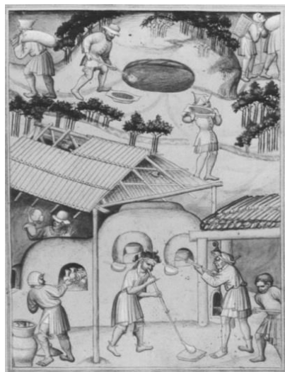
Figure 1 Representation of a Medieval Forest Glass hut.
