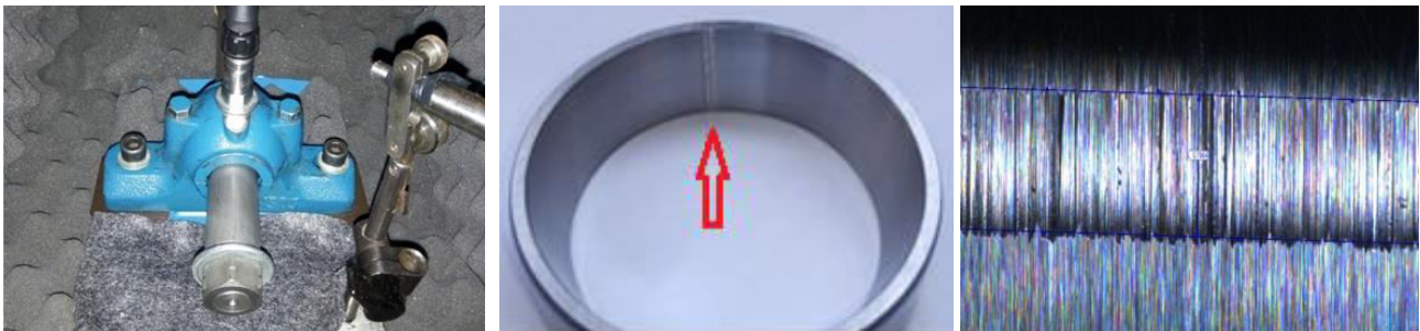
Figure 1 Outer ring (OR2) of the tapered roller bearing with grinding defect of 1.2492 mm (left) and its 50x enlarged image by Garant MM1-200 video microscope
