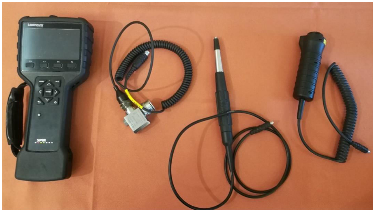
Figure 1 The measuring equipments (from left: Leonova Diamond – DIA 300 processing unit, SLD-144S vibration measuring unit, TRA73 shock pulse meter and TTP10 laser tacho/temperature meter )
