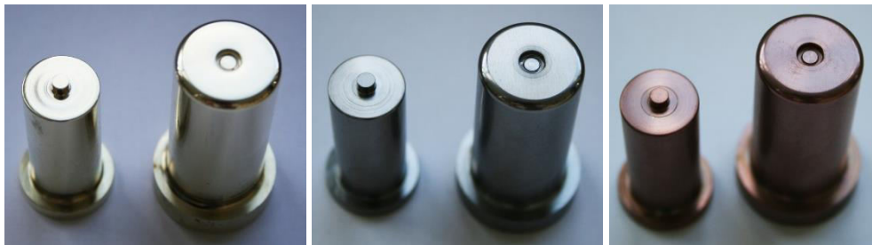
Figure 1 Punch and die of clinching tool: a) ZrN coating, b) CrN coating and c) TiCN MP coating
