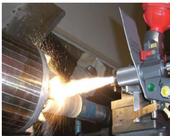
Figure 1 Rotor repair with cold spray process
