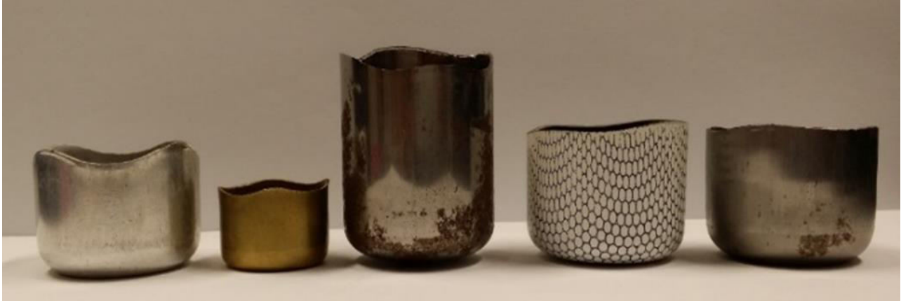
Figure 2 The earing represented after deep drawing
