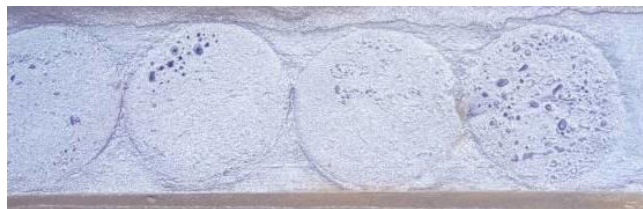
Figure 1 Gas defects caused by improper use of direct chills in steel casting
