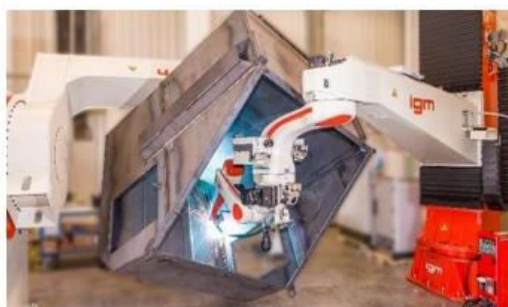
Welding robot system for waste containers
