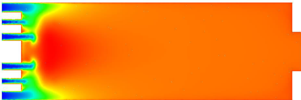
Figure 3 Temperature distribution (colour code: red 2440 K, blue 388 K)
