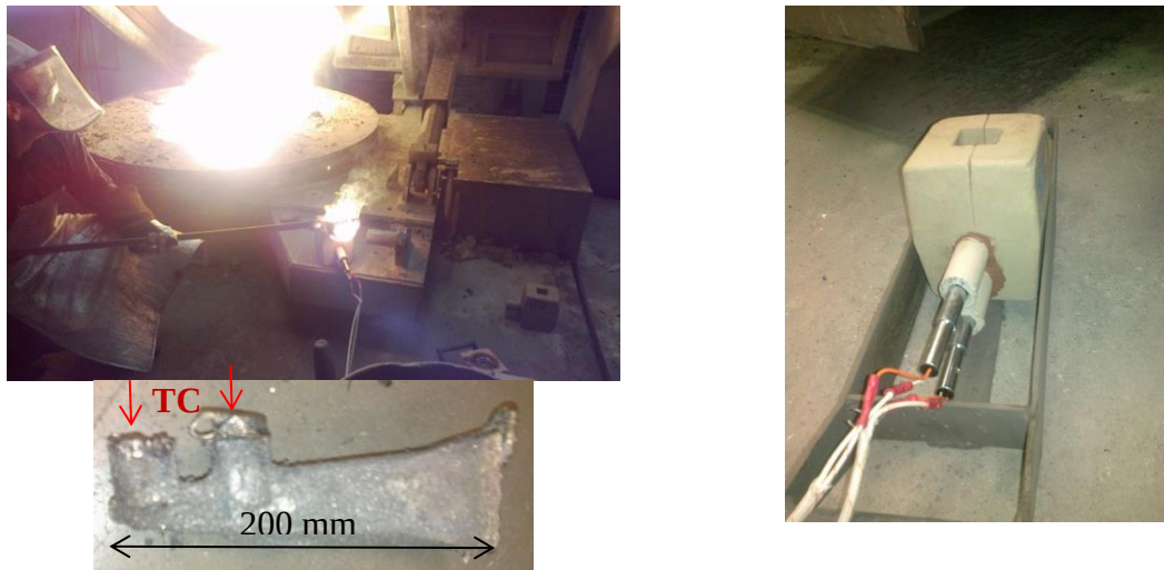
Fig. 1. Pouring the sand crucible and the wedge shaped sample with the thermocouples (TC) branch joints and the sand crucible with TCs
