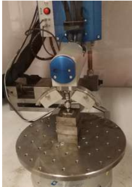
Figure 4. Centreless X-ray diffractometer with high speed rotation table
