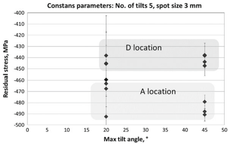
Fig. 6 Residual stress data in function of max tilt angle
