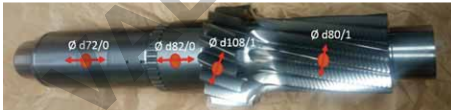
Fig. 1. Counter shaft. The points and the direction of the measured stress are indicated.
